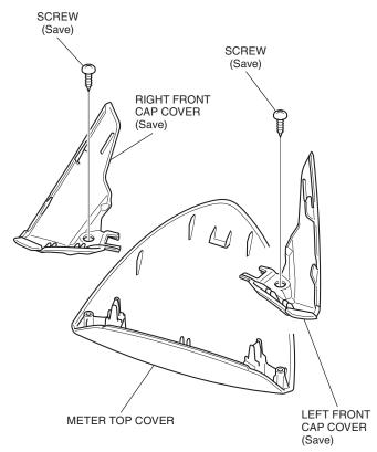
13. Install the meter top cover as shown.
