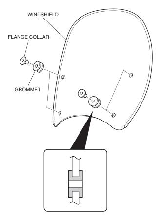
7. Temporarily install the windshield as shown.
