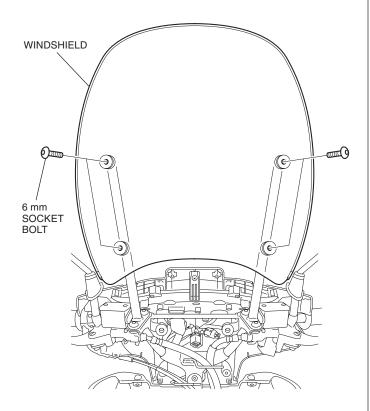
8. Tighten the loosely installed 8 mm socket bolts as shown.
