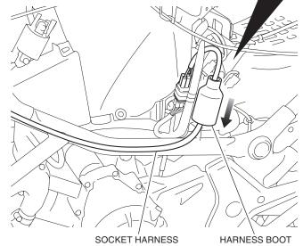
13. Secure each harness with the wire tie as shown.
