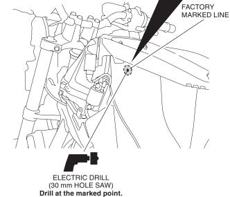
6. Install the ACC socket as shown.
