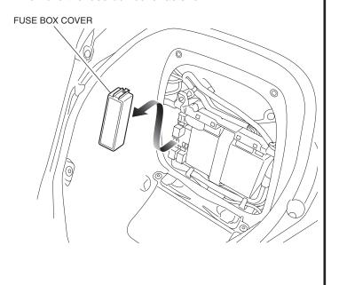
3. Install the relay and fuse in the position shown.
