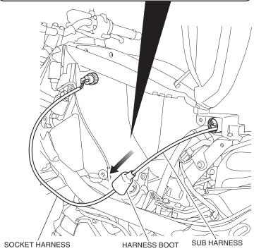
13. Secure the sub harness with the wire tie as shown.
