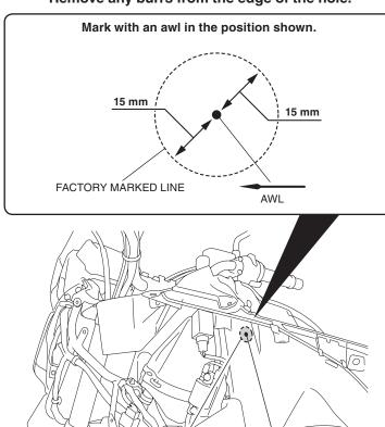
Install the ACC socket as shown.
