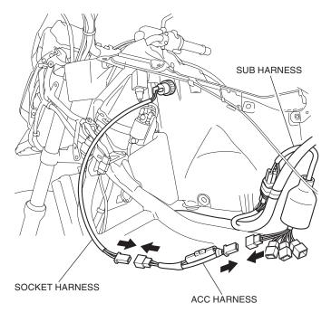
12. Cover the connectors with the harness boot as shown.
