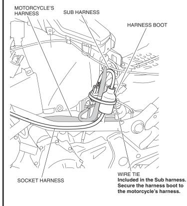
14. Bundle the socket harness and secure it with the wire tie as shown.
