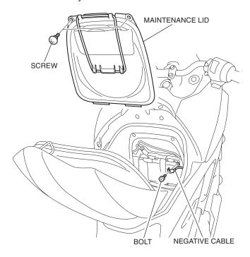
2. Remove the fuse box cover as shown.
