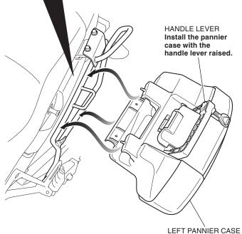
3. Lower the handle lever and lock the left pannier case by turning the key counterclockwise as shown.
