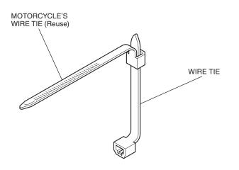
15. Secure the accessory socket harness with the wire tie as shown and put each harness.
