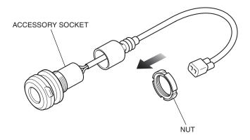
6. Assemble the accessory socket as shown.
