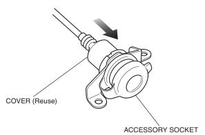
8. Install the assembled accessory socket as shown. <Right side>
