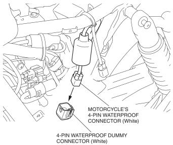
11. Install the dummy connector to the accessory socket sub harness as shown.
