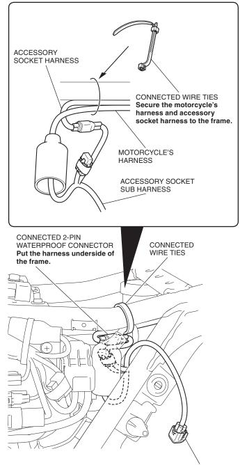
ACCESSORY SOCKET SUB HARNESS 16. Route the accessory socket sub harness as shown and put the connector.
