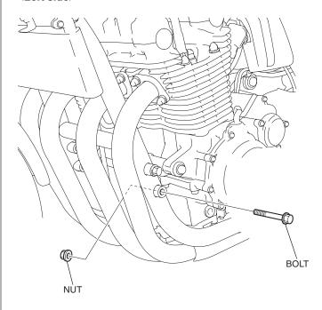
2. Loosely install the left side engine bar as shown.
