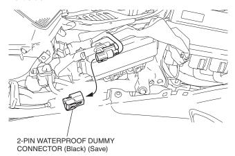
31. Remove the dummy connector as shown.
