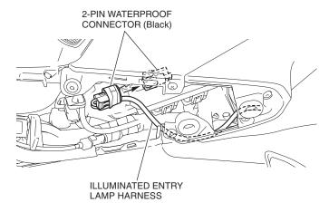
34. Secure the illuminated entry lamp harness with the wire tie.
