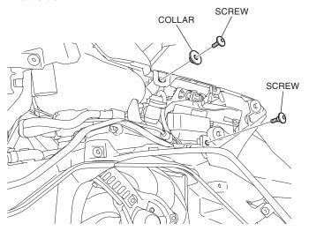
17. Remove the connector as shown.
