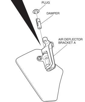
8. Install the pin as shown.
