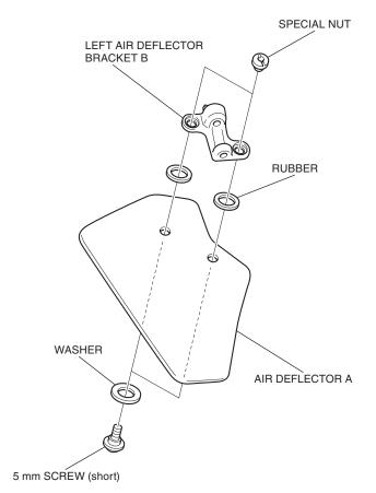
7. Install the air deflector bracket A as shown.
