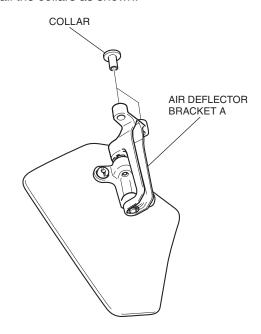
Install the assembled left air deflector A as shown.
