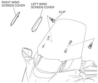
3. Remove the wind screen as shown.
