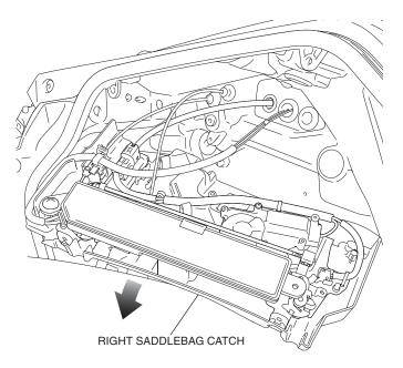
25. Remove the radio antenna as shown.
