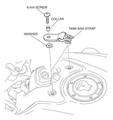
6. Install the tank bag on the fuel tank as shown.
