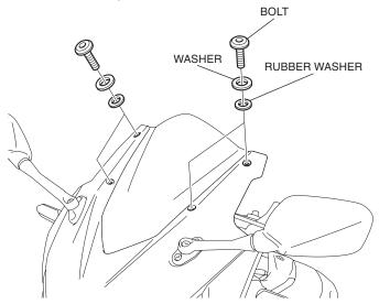
2. Remove the wind screen as shown.
