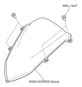
4. Install the well nuts as shown.
