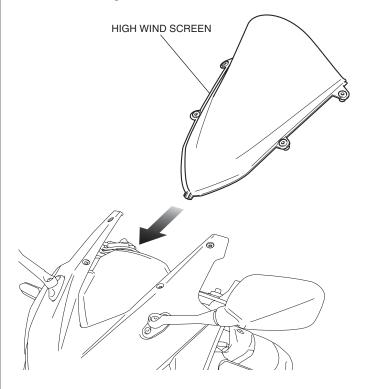
6. Install the parts as shown.
