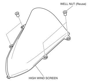
5. Install the high wind screen as shown.
