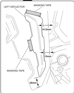
3. Peel off the adhesive backing on the left deflector as shown.
