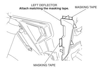
5. Remove the adhesive backing as shown.
