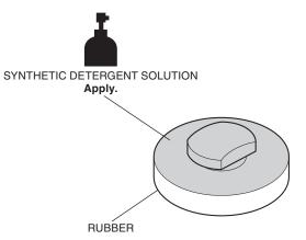
2. Install the rubber in the position shown.
