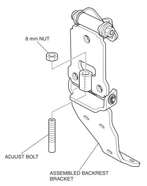
10. Install the special nuts as shown.
