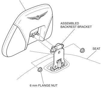
17. Tighten the loosely installed 6 mm flange nuts securely.
