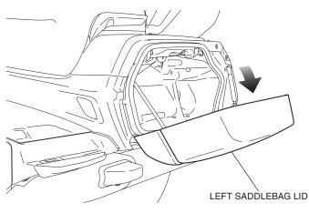
2. Remove the left side cover as shown, and disconnect the negative (-) cable of the battery.
