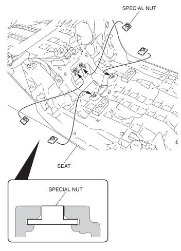
11. Insert the assembled backrest bracket as shown.
