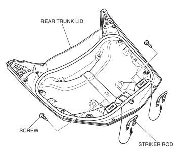
27. Remove the inner trunk lid as shown.
