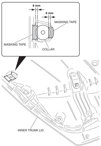
37. Install the inner trunk lid to the trunk lid as shown.
