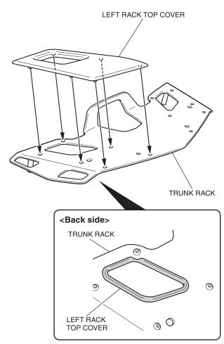
40. Apply synthetic detergent solution to the position shown.
