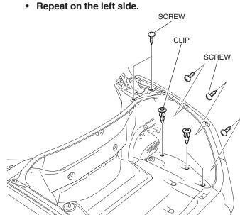
15. Remove the right trunk side cover as shown.Repeat on the left side.
