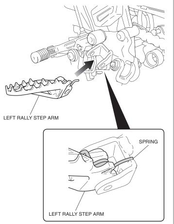
7. Install the pivot pin and split pin as shown.
