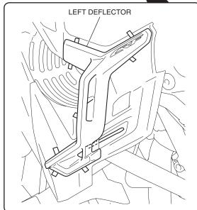
6. Remove the adhesive backing as shown.
