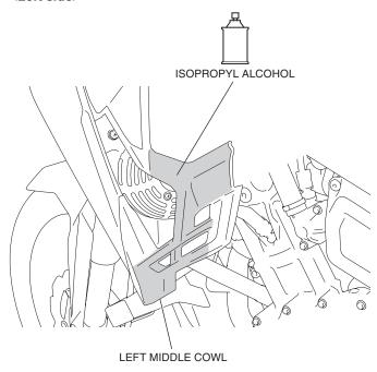
4. Peel off the adhesive backing on the left deflector as shown.
