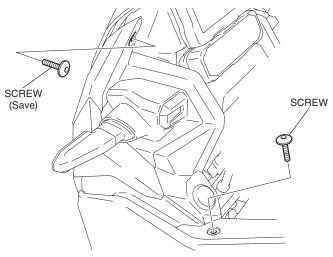
2. Clean the surface of the area shown using an isopropyl alcohol.
