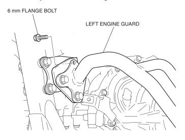
23. Loosely install the left engine guard as shown.
