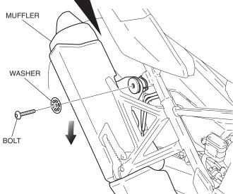
16. Remove the parts as shown.
