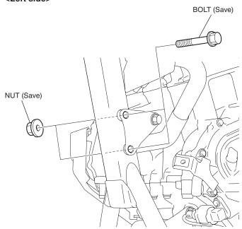
17. Remove the bolt as shown.
