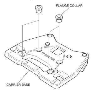
4. Install the carrier base as shown.
