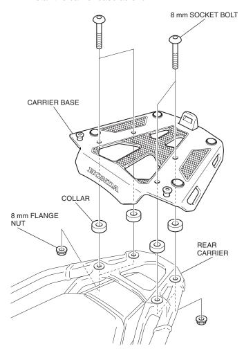
3. Refer to the Genuine Accessory User's Guide that comes together with the top box, and install the top box according to the instruction.
