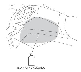
5. Attach the protection film to the fuel tank as shown.
