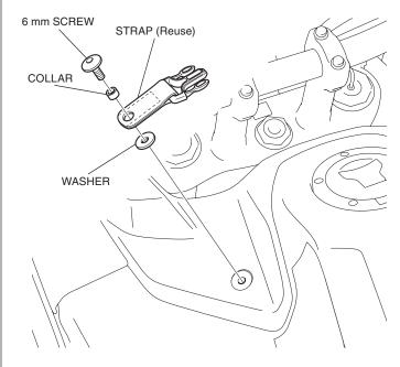
9. Install the tank bag on the fuel tank as shown.
