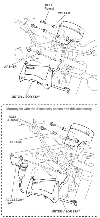
4. Loosely install the bolt as shown.
