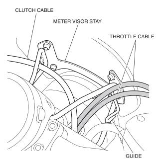
8. Move the handlebar right and left, and check that this accessory is not interfere with the motorcycle parts.
