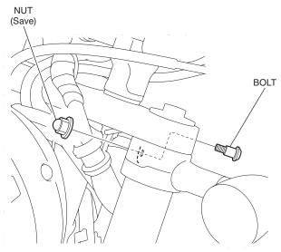
3. Loosely install the meter visor stay as shown.
