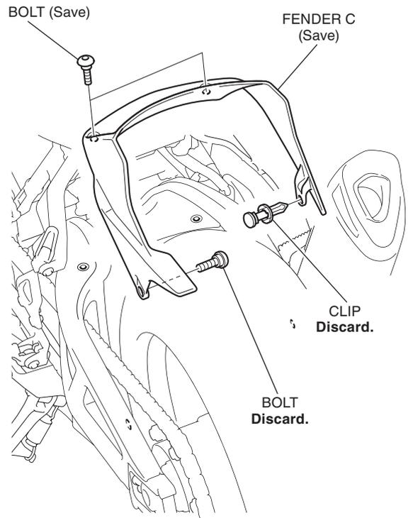
2. Install the rear fender C as shown.
