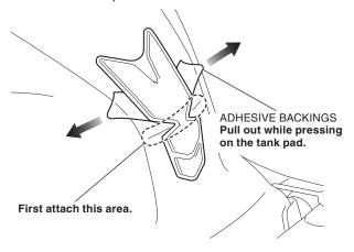
5. Attach the tank pad while pressing down radially as shown.
