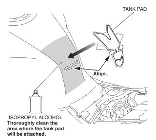
4. Attach the tank pad as shown.
