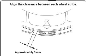
4. Press firmly on the installed wheel stripes to adhere.
