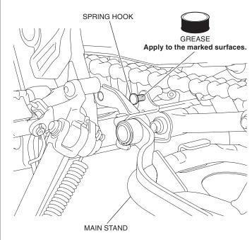
12. Install the spring plate as shown.
