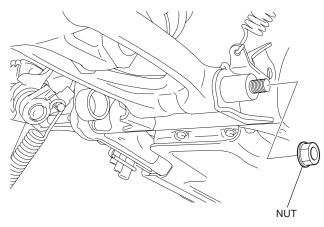
2. Apply synthetic detergent solution to the position shown.
