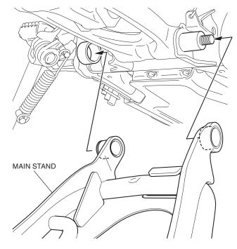
7. Install the nut in the reverse order of removal.
