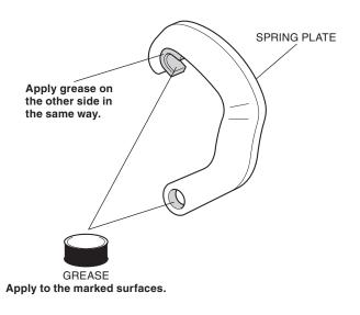
10. Install the springs to the spring plate as shown.
