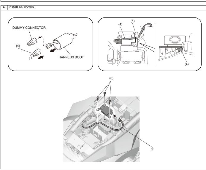
5. Install the motorcycle's parts in the reverse order of removal.
