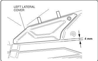
6. Remove the adhesive backing as shown.
