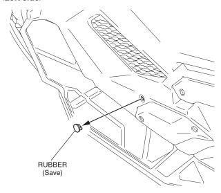
Clean the surface of the area shown using an isopropyl alcohol.
