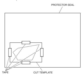
5. Cut both the template and protector seal together along the dotted line as shown.
