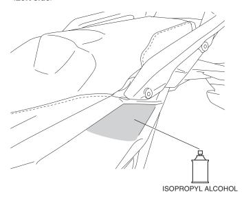
7. Attach the protector seal to the left rear cowl as shown.
