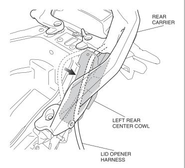
14. After route the lid opener harness, install the screw as shown.
