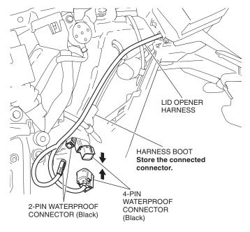
17. Secure the lid opener harness with the wire tie as shown.
