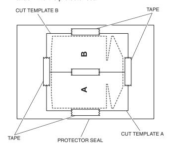
3. Cut both the templates and protector seal together along the dotted line as shown.
