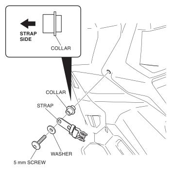
7. Open the seat, and route the adjust strap as shown.
