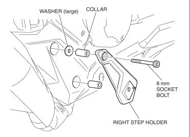
4. Loosely install the right step bracket as shown.
