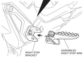
11. Install the joint pin and split pin as shown.
