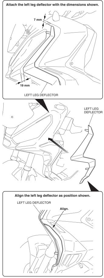
4. Remove the adhesive backing as shown.
