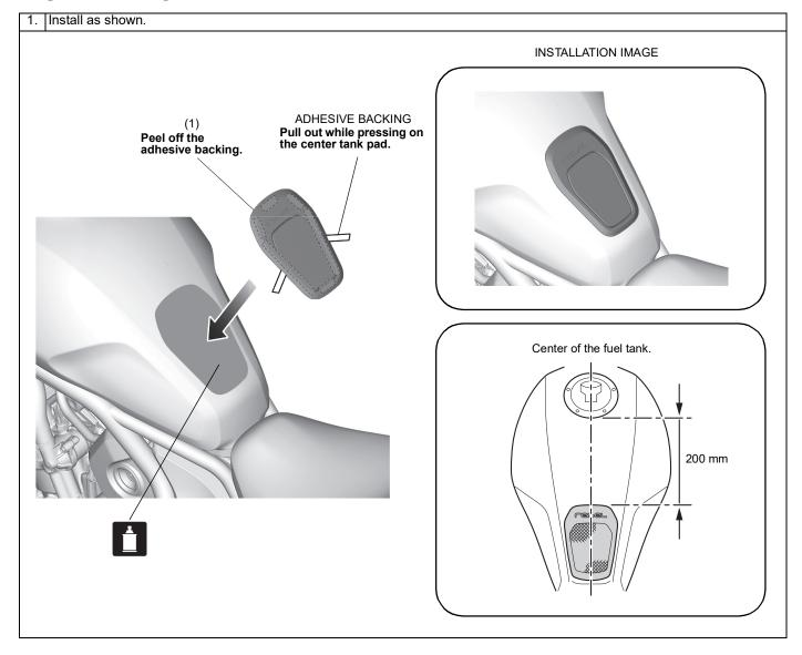
2. Apply adequate pressure to the center tank pad.
