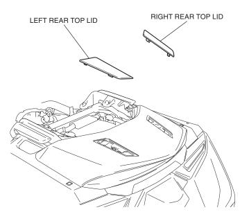
8. Remove the parts as shown.
