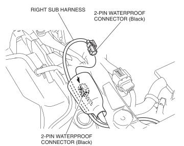
31. Secure the right sub harness with the wire ties as shown.
