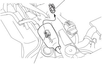
2-PIN WATERPROOF CONNECTOR (Black) 30. Connect the right sub harness as shown.
