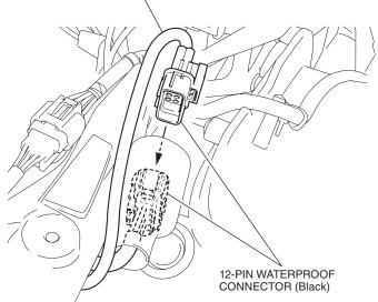
36. Secure the left sub harness with the wire tie as shown.
