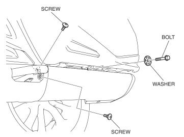
3. Loosen the bolt, then remove the left muffler as shown.
