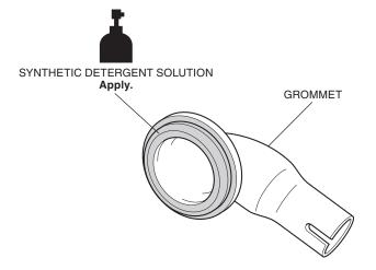
27. Install the grommets as shown.
