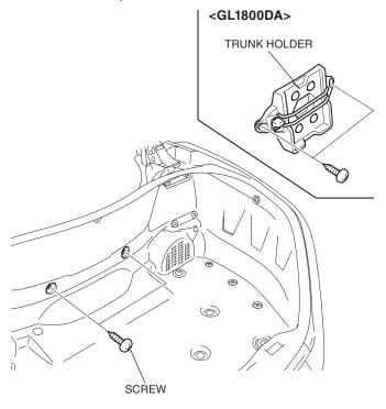
12. Remove the front trunk lower panel as shown.
