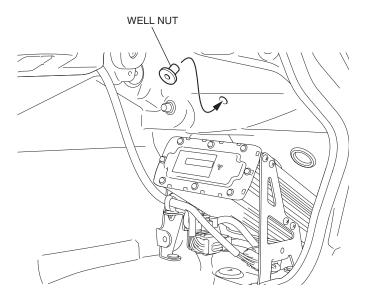
49. Clean the surface of the area shown using an isopropyl alcohol.
