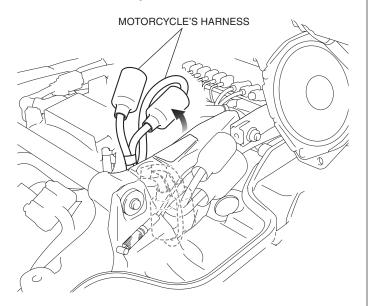
37. Disconnect the connector as shown.
