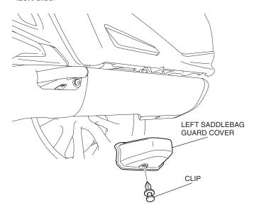
2. Remove the parts as shown.
