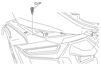
18. Remove the rear fender as shown.
