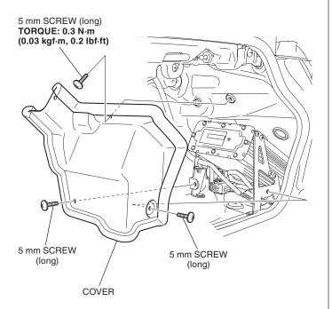
52. Install the 5 mm screw as shown.
