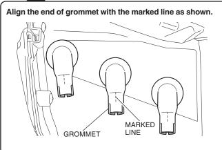
28. Install the hole plug as shown.
