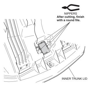
3. Mark the trunk inner lamp harness in the position as shown.
