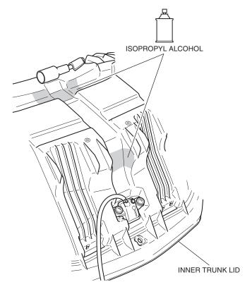
7. Connect the trunk inner lamp harness as shown.
