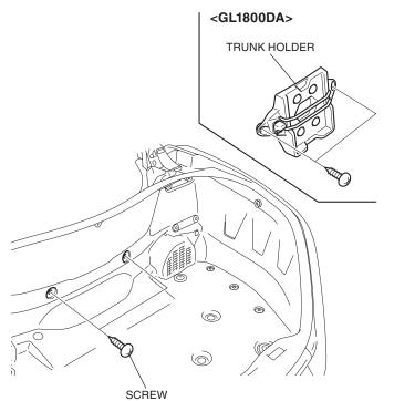
13. Remove the front trunk lower panel as shown.
