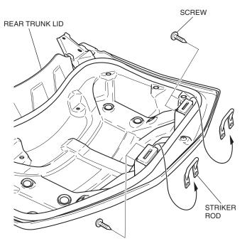
18. Remove the inner trunk lid as shown.
