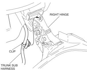
28. Route and secure the trunk sub harness as shown.
