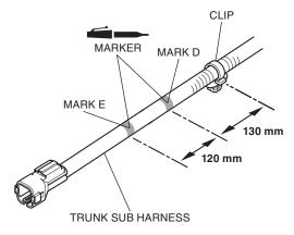
23. Clean the surface of the area shown using an isopropyl alcohol.
