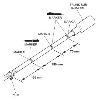
22. Mark the trunk sub harness in the position as shown.
