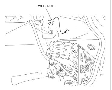
46. Clean the surface of the area shown using an isopropyl alcohol.
