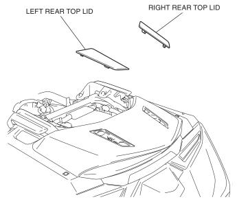
11. Remove the parts as shown.
