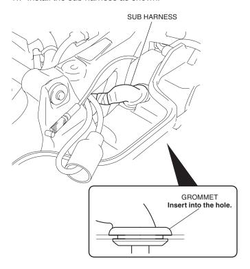
42. Secure the left sub harness with the wire tie as shown.
