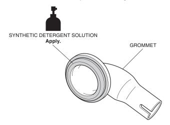
24. Install the grommets as shown.
