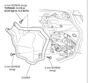
49. Install the 5 mm screw as shown.
