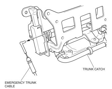
21. Remove the trunk sub assembly as shown.
