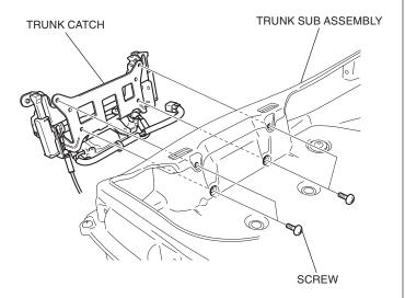
20. Remove the emergency trunk cable as shown.
