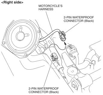
17. Disconnect the connector and remove the center trunk lower cover as shown.
