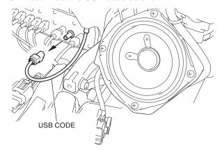
16. Disconnect the connector as shown.
