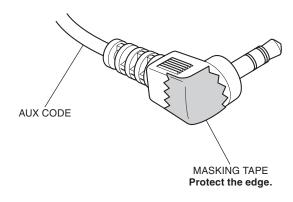
25. Apply synthetic detergent solution to the position shown.
