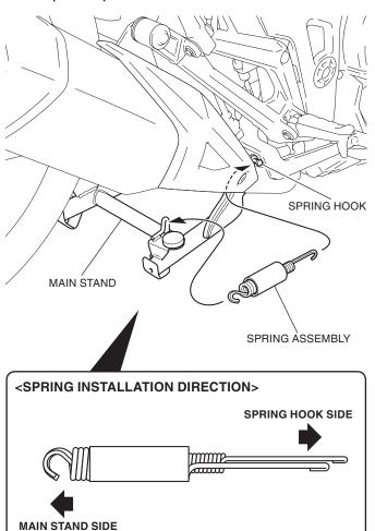
If the spring assembly is too hard to install, remove the main stand shaft. First hook the spring assembly, then install the main stand shaft.
