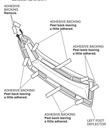
14. Peel off the adhesive backings on the left foot deflector as shown.
