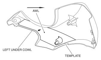
4. Remove the templates. Drill at the marked point shown using an electric drill.
