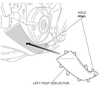
16. Remove the adhesive backings as shown.
