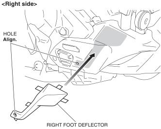
10. Remove the adhesive backings as shown.
