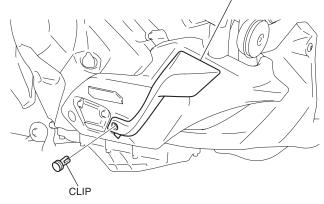
13. Clean the surface of the area shown using an isopropyl alcohol.
