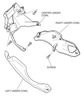
Cut and attach the templates to the under cowls and mark them using an awl as shown.
