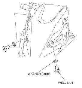
4. Loosely install the high wind screen as shown.
