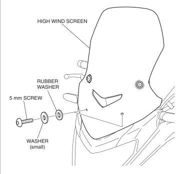
6. Tighten all loosely installed parts securely.
