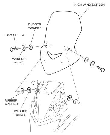
5. Loosely install the 5 mm screws as shown.
