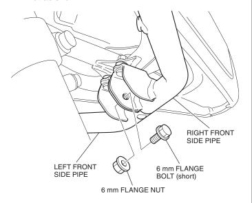
6. Tighten all loosely installed hardware to the specifications in the torque chart.
