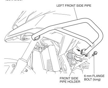
2. Loosely install the left front side pipe as shown.
