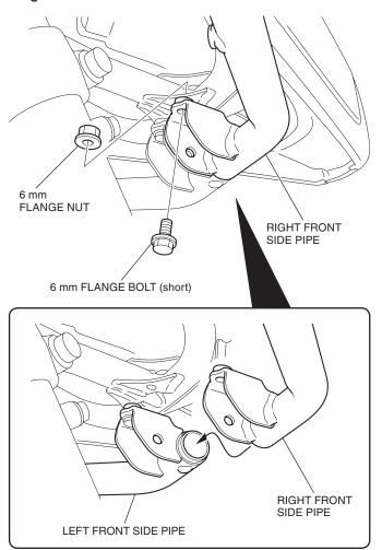
5. Install the 6 mm flange bolt (short) and 6 mm flange nut as shown.
