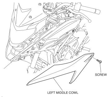
7. Remove the left front side cowl as shown.
