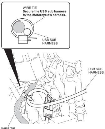
WIRÉ TIE Secure the USB sub harness to the motorcycle's harness.
