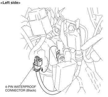
15. Remove the dummy connector as shown.
