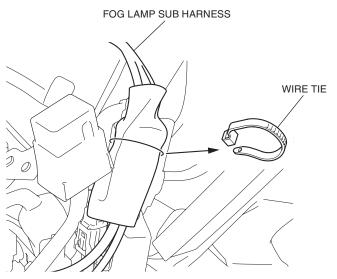
14. Remove the connector as shown.
