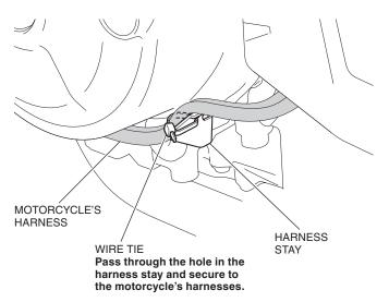
12. Mark the gear change switch harness in the position shown.
