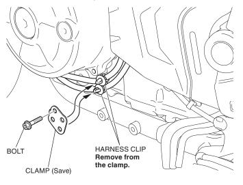
9. Remove the harness clips as shown.
