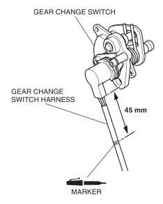
13. Loosely install the shifter unit stay to the gear change switch as shown.
