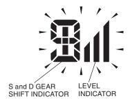
S gear shift indicator, level indicator and D gear shift indicator blink alternately 5 seconds after deregistration is completed.
