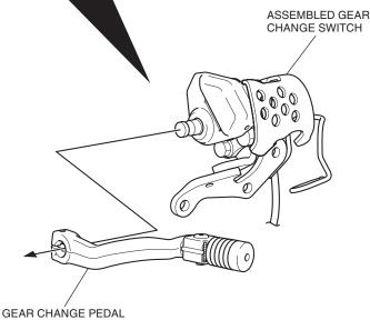
18. Install the 6 mm flange bolt as shown.
