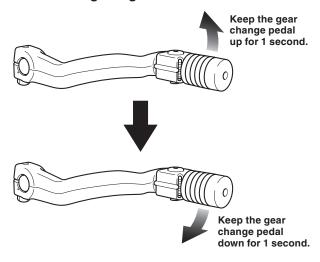
S gear shift indicator, level indicator and D gear shift indicator blink alternately after the registration is completed.
