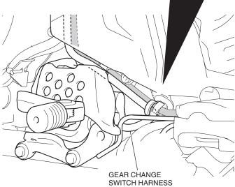
23. Route and connect the gear change switch harness as shown.
