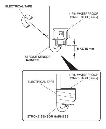
15. Install the assembled stroke sensor as shown.
