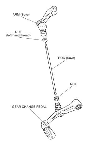
5. Loosely install the tie rod bolt as shown.
