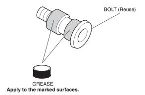
17. Filling grease to the position shown.
