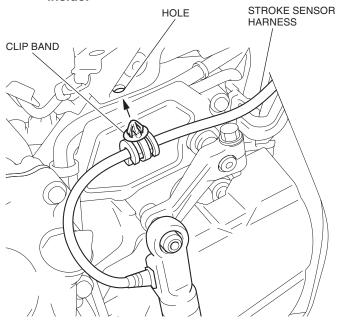
23. Secure the stroke sensor harness with the wire tie as shown.
