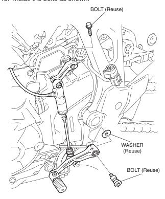
19. Tighten the loosely installed parts securely to the dimension shown.
