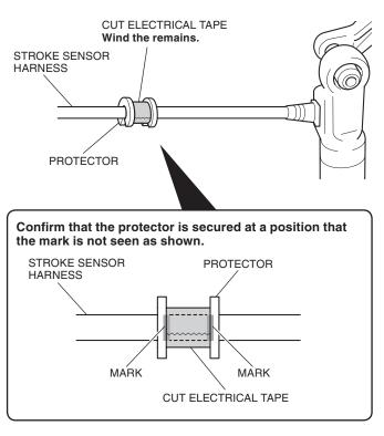
14. Secure the stroke sensor harness in the position of the dimension shown.
