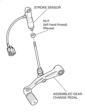
7. Install the gear change arm as shown.
