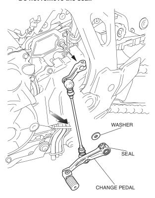
4. Remove the rod and arm as shown.
