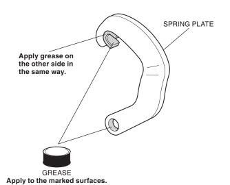
10. Install the springs to the spring plate as shown.
