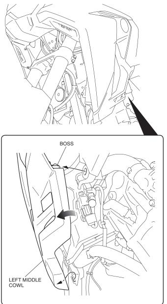
3. Clean the surface of the area shown using an isopropyl alcohol.
